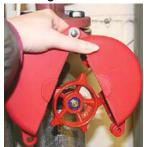
Gate valve covers are a simple, low cost and highly effective way to prevent unauthorised operation of valves. Valve covers consist of two flattened half moons that slip over the valves hand wheel and completely cover it. Once locked, the cover rotates freely around the hand wheel preventing operation.
